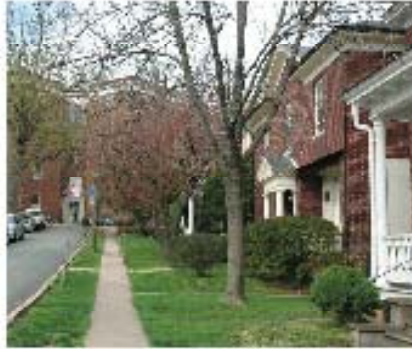
Altamont St. 4'-0" Planting Strip w/3'-0" sidewalk
